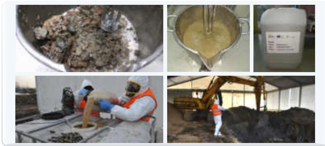
Figure 8 Application of the produced microorganisms to the mesocosms and to the biopile
