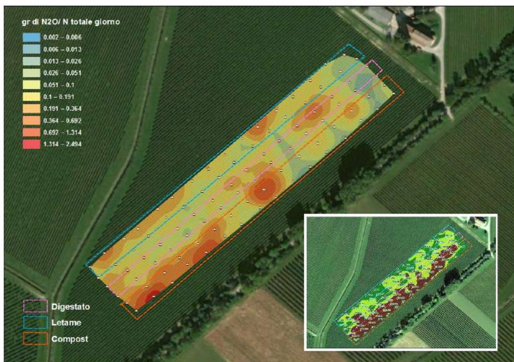
Figure 13. Bosco del Merlo, march 2017. Isoflux map of nitrous oxide emissions. The vigour map is shown in the box below right
