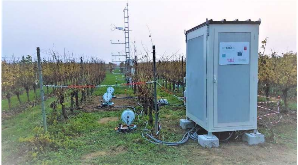
Figure 8. The picture shows the instrumentation used for the continuous monitoring of GHG fluxes from soil planted to grapevines at the Bosco del Merlo site. Sensors were installed near the Eddy Covariance station.
