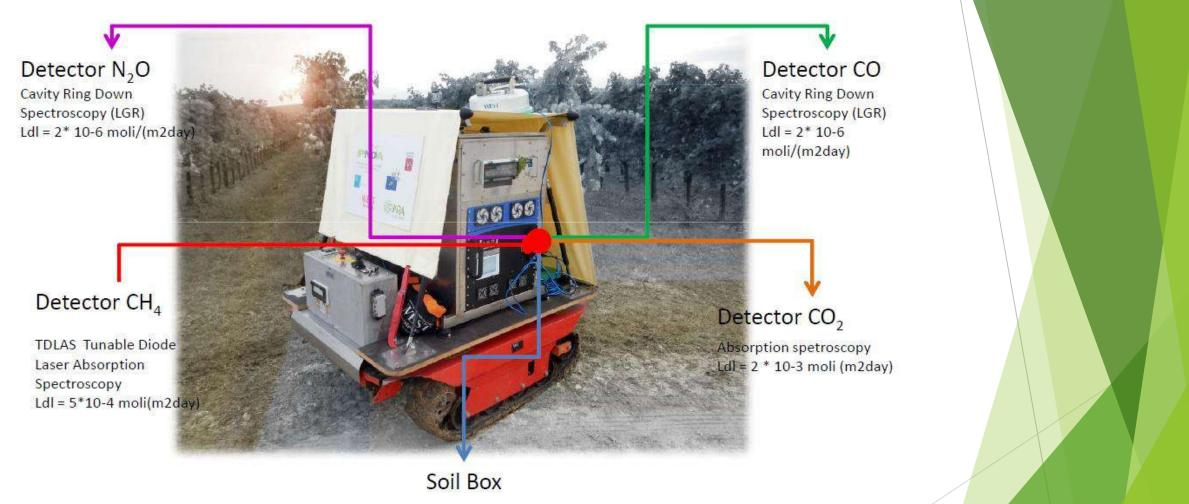
Mobile instrumentation, developed as part of a previous LIFE+ IPNOA project (LIFE11 ENV / IT / 000302), which consists of an electric tracked vehicle on which the <u>analyzers of carbon dioxide</u>, <u>nitrous oxide</u>, <u>methane</u> <u>and carbon monoxide</u>. The flows emitted from the soil are quantified using the <u>methodology of the non-</u><u>stationary static accumulation chamber</u>
