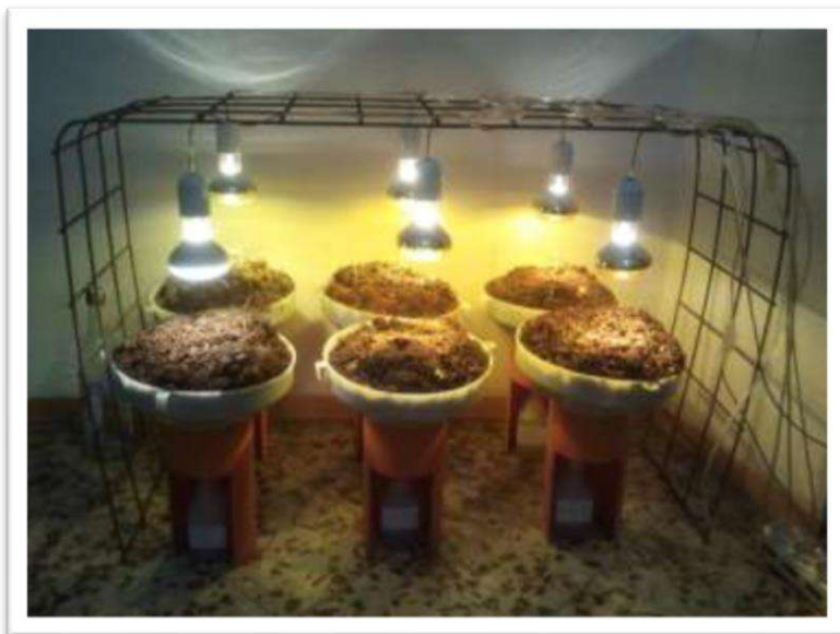
Figure 7. Berlese-Tullgren selector for the sampling of the soil microfauna and QBS-ar index calculation
