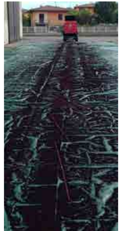
Figura 3. Free-surface distribution assessment test.
